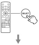
Press the Cursor button ( $\wedge$ / $\vee$ ) to adjust the value of the selected item, and then press the SELECT button.
